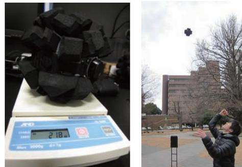
we propose a novel concept called VolVision that encompasses using a camera to reconstruct 6DoF unconstrained motion. "VolVision" is designed to handle imagery falling, tossed or thrown cameras. And VolVision also allows users to reconstruct dynamic images and generate a 3D-mapped scene from image
