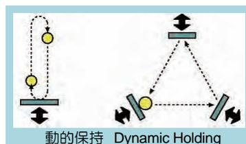
In order to achieve faster and more dexterous manipulations, we are proposing a strategy called "dynamic holding." In the dynamic holding condition, an object is held in a stable condition while the object is
