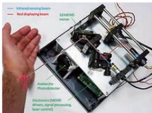
The 'Smart Laser Projector' (SLP) is a modified laser-based projector capable of displaying graphics on a variety of non-prepared surfaces, while simultaneously using the beam (at
