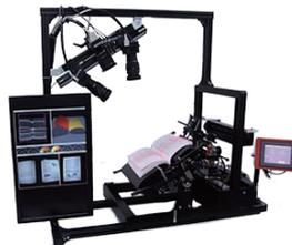
BFS-Auto can achieve high-speed and high-definition book digitization at over 250 pages/min using the original media format. This performance is realized by three key points: high-speed fully-automated page flipping, real-time 3D recognition of the flipped pages, and high-accuracy restoration to a flat document image.
