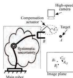
Figure 1. The proposed dynamic compensation concept
