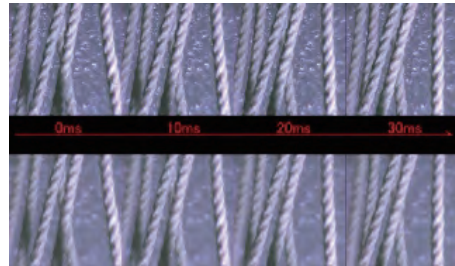
Figure 2. Results of DOF Extension (top: images synthesized by focus stacking; bottom: unsynthesized images).
