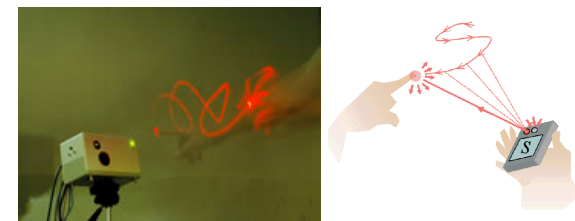
figure 5. The Smart Laser Scanner is able to track fingers and gestures in 3-space without using a camera.
