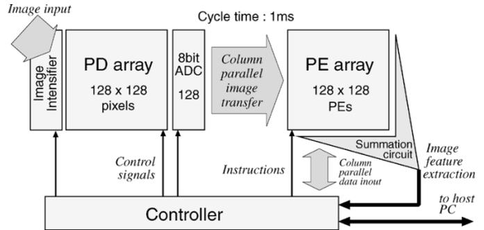
Fig. 6. Block diagram of I-CPV system.
