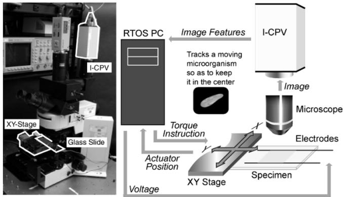
Fig. 4. System configuration.
