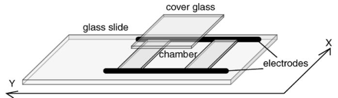
Fig. 7. Electrical stimulus input device.
