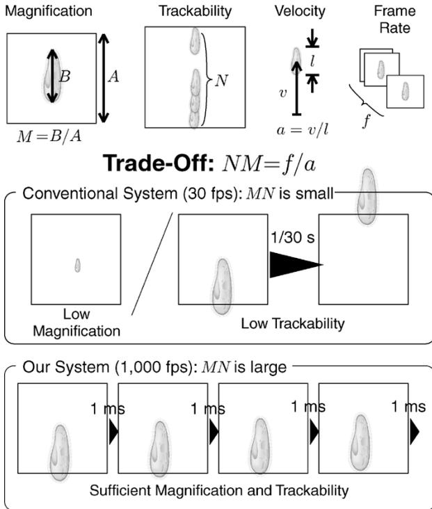
Fig. 3. Tradeoff between magnification and trackability in microscopic tracking.
