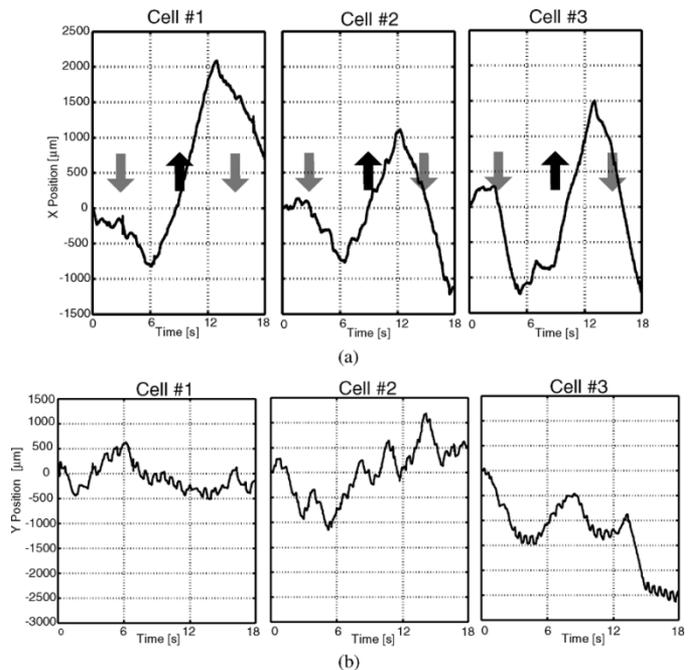
Fig. 12. (a)  $X$  position (parallel to the electric field) of cells in the open-loop control experiment. Arrows indicate the direction of the applied electric field. (b)  $Y$  position (perpendicular to the electric field) of cells in the open-loop control experiment.
