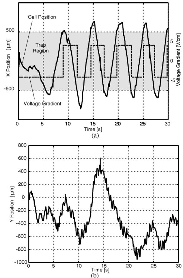
Fig. 14. (a) Applied voltage (dashed line) and  $X$  position (parallel to the electric field) of a cell (solid line) in the closed-loop control experiment. The shaded region is the bounded region for trapping. (b)  $Y$  position (perpendicular to the electric field) of a cell in the closed-loop control experiment.
