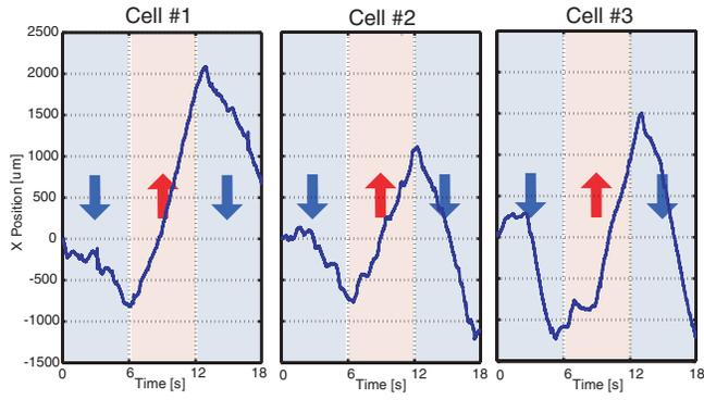
Fig. 9.  $X$  position (parallel to the electric field) of cells in feedforward control experiment. Arrows indicate the direction of the applied electric field.
