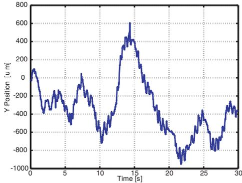
Fig. 14.  $Y$  position (perpendicular to the electric field) of a cell in feedback control experiment.
