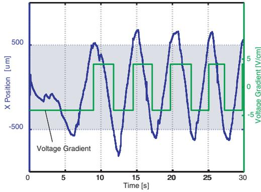
Fig. 13. Applied voltage (green) and  $X$  position (parallel to the electric field) of a cell (blue) in feedback control experiment. The shaded region is the bounded region for trapping.
