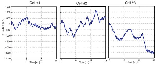
Fig. 10.  $Y$  position (perpendicular to the electric field) of cells in feedforward control experiment.
