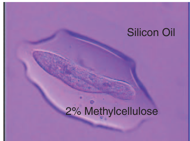
Fig. 5. A cell trapped within a droplet. Monitored with a color CCD camera (Hitachi, KP-D).
