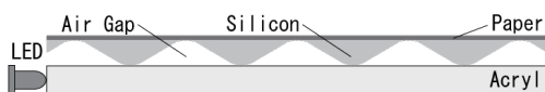
図2 FTIR 装置 (アクリル・LED・膜 (Compliant surface)) Fig.2 FTIR device (Acrylic Membrane (Compliant surface)).
