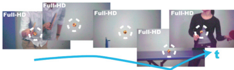
図2 卓球の1msオートパン・チルト映像(500fpsフルハイビジョン) Fig.2 Auto Pan-Tilt image sequence of a pingpong game. (500fps, Full-HD)
