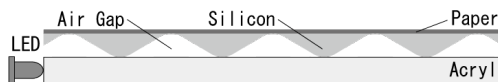
図 2 FTIR 装置 (アクリル・LED・膜 (Compliant surface)) Fig.2 FTIR device (Acrylic Membrane (Compliant surface)).
