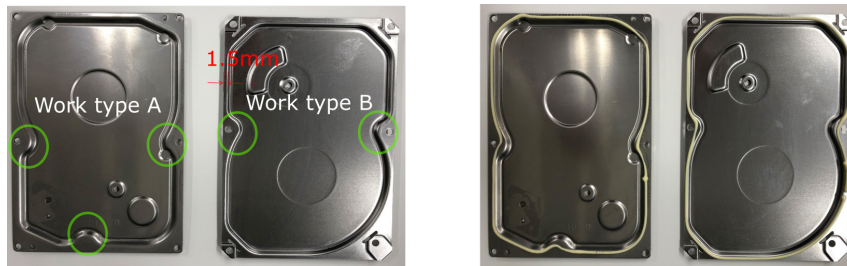
Fig.2 working target before and after dispensing
